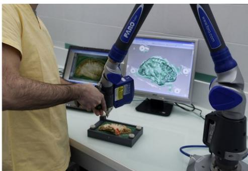
**Fig. 2.** Laser scanner. The laser scanner is composed of an articulated two-segment arm, whose tip displacement is recorded precisely and transferred to an attached personal computer. Surface information was mostly obtained from a laser pointer, but also from a mechanical probe, both attached to the arm tip. For surface acquisition, the laser was displaced onto the anatomical specimen, and a mesh was computed and displayed online from impacts of the beam on the surface.
